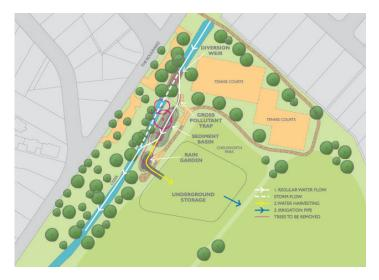
Modelling indicates that more than 30 Olympic swimming pools worth of stormwater will be harvested per annum (approximately \$200,000 worth of potable water). The storage has a capacity for 80 mega litres of water and improvements to the irrigation infrastructure at Chelsworth Park and the Ivanhoe Golf Course has occurred.
